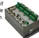
Master Control Module for VF1-75, JR1000 and the JD400
