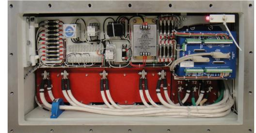
Mounted in explosion proof box with VF-1200 tram drive.
