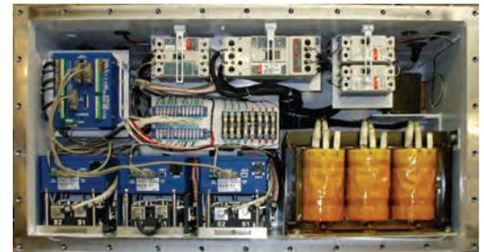
Three drive system for shuttle cars
