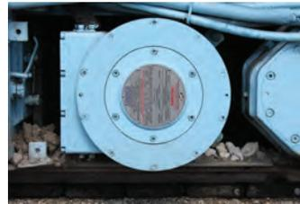
TM1200 continuous miner tram motor installed
