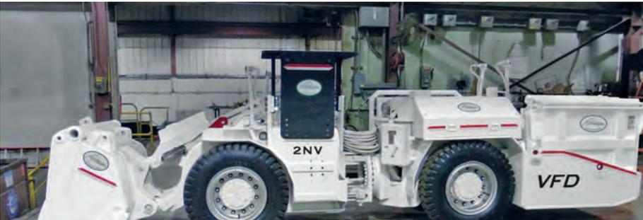
*Before and After - images of an LHD rebuild where electric drives and battery electric specialist Saminco converted the machine from diesel to battery power for the lead rebuilder, client Highland Machinery*
